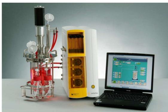
Figure 1. Sartorius-stedim Biostat<sup>®</sup> A Plus fermentation system
