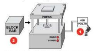
In the above example, a padlock (1) is used to lockout the electrical box and a blocking bar (2) is used to prevent the press weight from dropping (releasing of stored energy).
