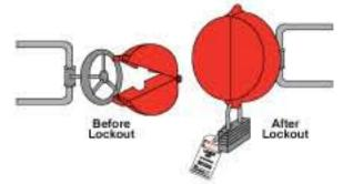
A Safetee Donut™ is a device that can be used to lockout round valve handles of varying diameters. The device loosely encases the valve handle, preventing access and turning of the handle.
