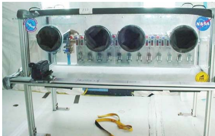
Fig. 4 Double-walled Lexan glove box with two sets of industrial strength rubber gloves. The glove box is shown in this picture with a previously flown experiment and only one camera mounted.
