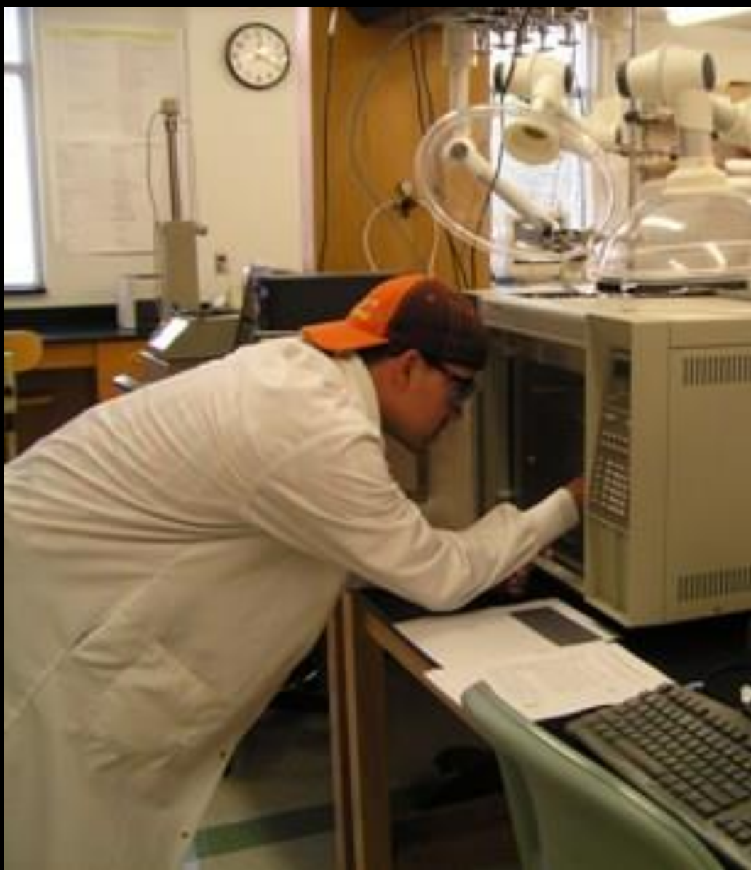
2007: Josh Locklear installing a column on a gas chromatograph
